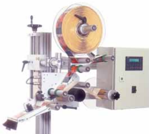
Label applicator L100. For pre-printed labels. On "Height adjustment" stand.
